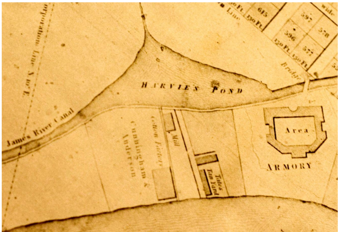
(Figure 16.) This detail from the 1835 Bates Atlas illustrates the large Harvie Pond, also known as the Penitentiary Basin, before the sides of the pond were shored up with stone later that decade. The south bank of the canal at this location served as a dam to hold back the water from the creeks and springs that fed Harvie's Pond. (Source: Library of Virginia)
