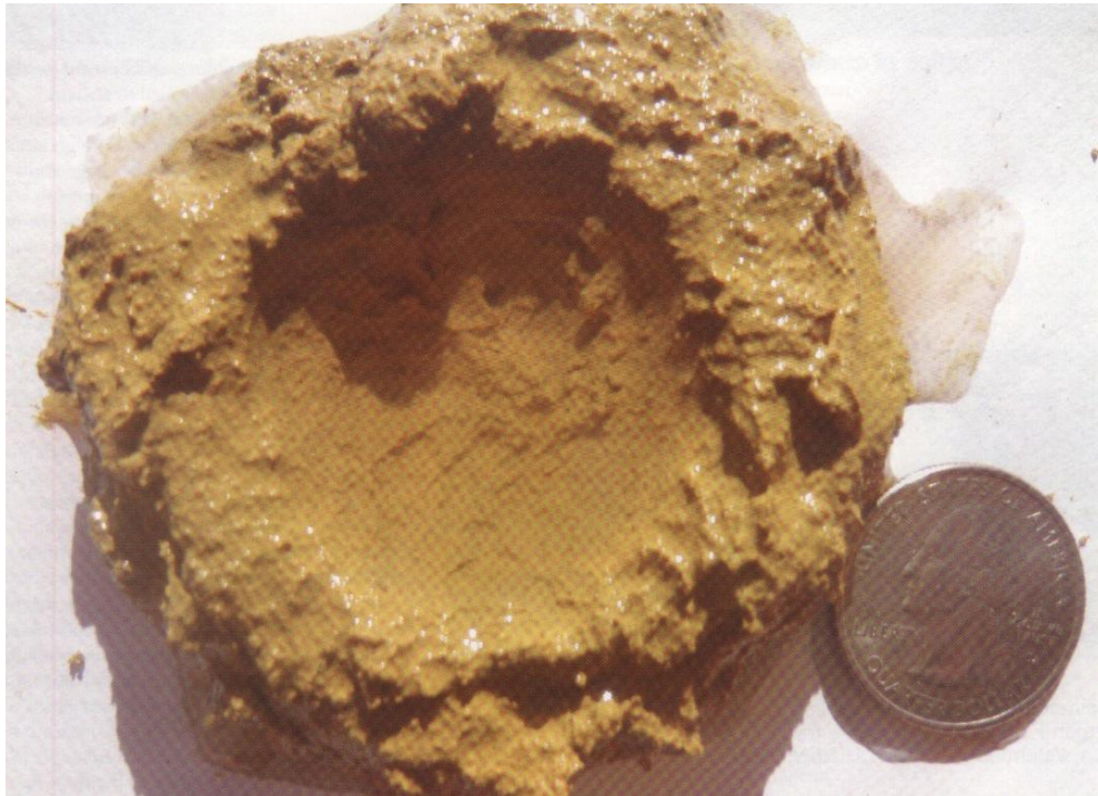
(Figure 36.) Canal authority, Dr. Bill Trout, sampled the clay from the canal tow path when the canal was cut in order to build the 2 nd Street Connector in 2012. He demonstrated that puddling this clay made it leak proof. (Source: The Tiller , publication of the Virginia Canals and Navigations Society, Vol. 34-1, 2012, pages 8-9)
