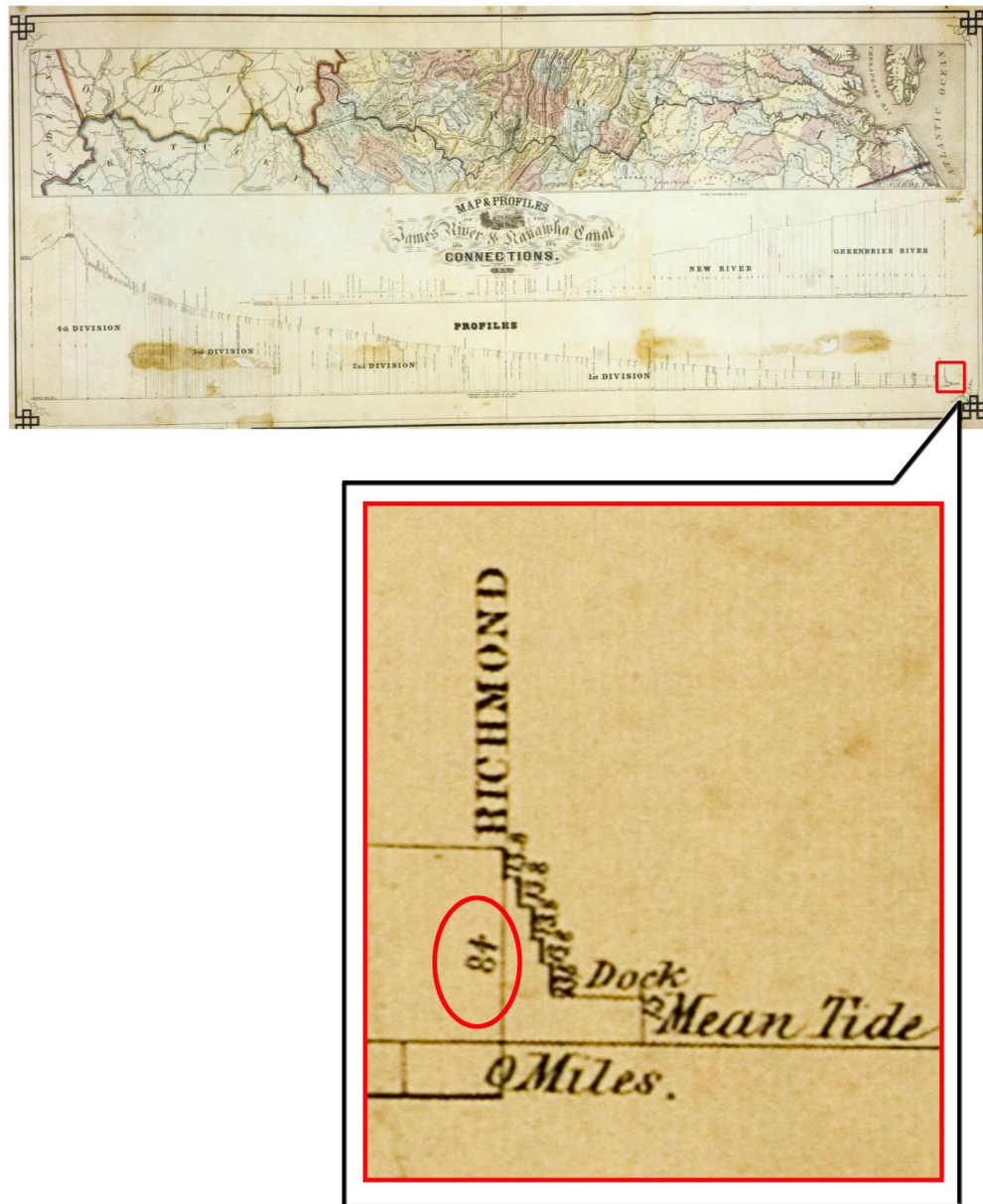
(Figure 30.) This very detailed 1857 Board of Public Works map indicates that the water elevation of the canal at the Richmond level was 84 feet above "Mean Tide." (Source: Edward Lorraine, Map and profiles of the James River and Kanawha Canal and its connections , BPW 496 (9), 1857, Library of Virginia)
