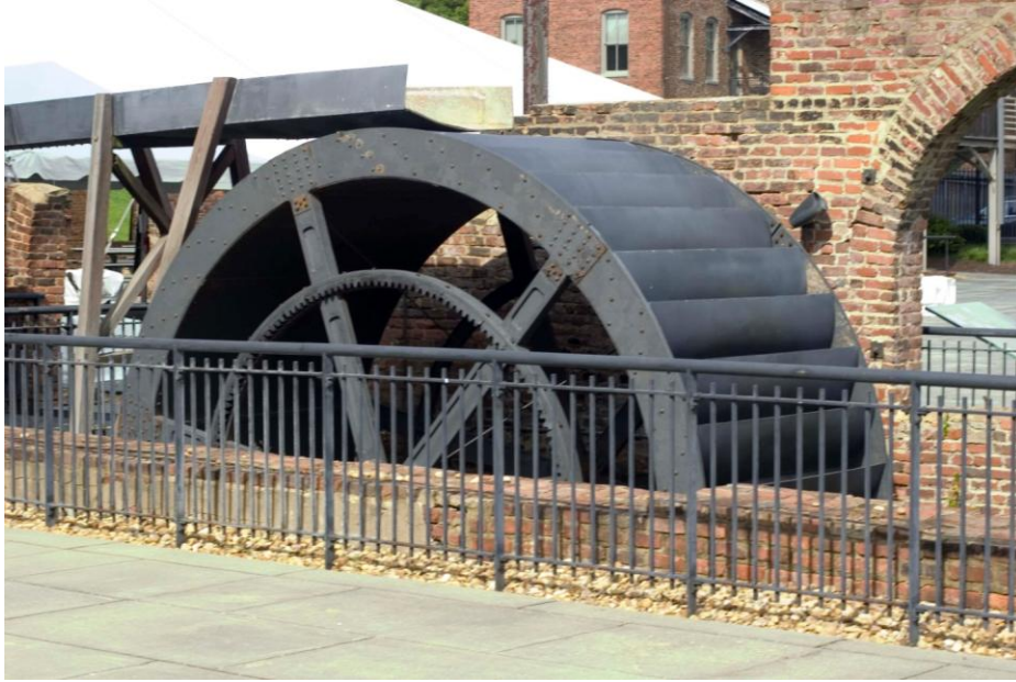
(Figure 60.) This is a replica of the overshot wheel at Tredegar that was powered by water from the James River and Kanawha Canal. With a 50 foot drop from the canal to the James River, each water race could power up to three mills in sequence. Widening the canal in 1838 greatly increased available water volume. (Source: OHHIC)
