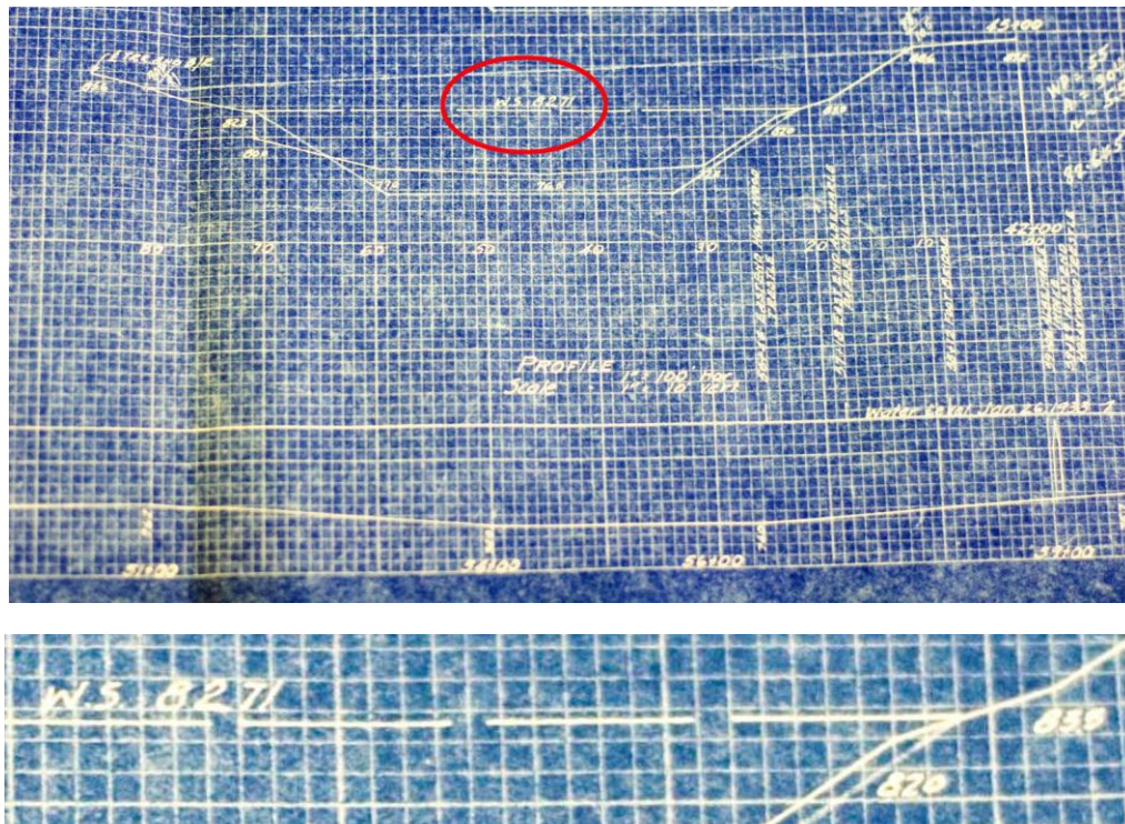
(Figure 34.) Trimble survey (and detail) documenting the water surface in the canal at 82.71 feet at Tredegar in 1933. (Source: Tredegar Papers, Box 31, Tube #1, Accession Number 23881, 24808, Library of Virginia)
